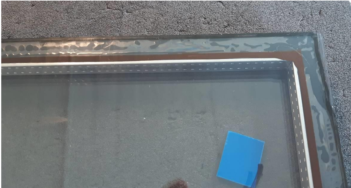
Specimen as received with sealant adhesion problem (not used for tests).
